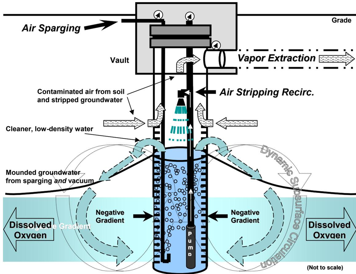
Exhibit-2 Synergistic subsurface effects of a typical ART well
